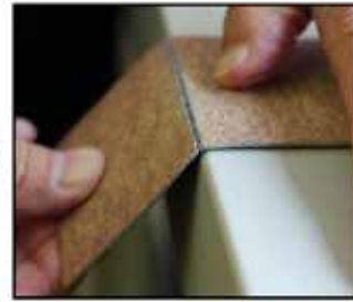
3. Fit the notch to a square corner and move the end up and down to separate it.
