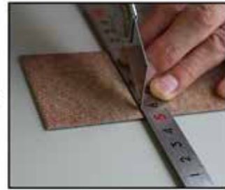
2. Make a notch that is more than half the thickness.
